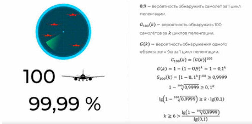
Figure 2 Bernoulli scheme for radar aircraft detection
